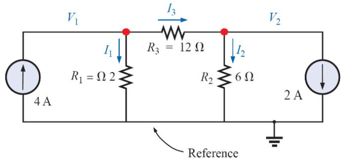
$$\frac{7}{12}V_1 - \frac{1}{12}V_2 = +4 \implies 7V_1 - V_2 = 48$$
