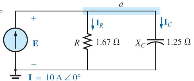
$$\begin{aligned} Z_T &= \frac{Z_R Z_C}{Z_R + Z_C} = \frac{(1.67 \Omega \angle 0^\circ)(1.25 \Omega \angle -90^\circ)}{1.67 \Omega \angle 0^\circ + 1.25 \Omega \angle -90^\circ} \\ &= \frac{2.09 \angle -90^\circ}{2.09 \angle -36.81^\circ} = \mathbf{1 \Omega \angle -53.19^\circ} \end{aligned}$$
