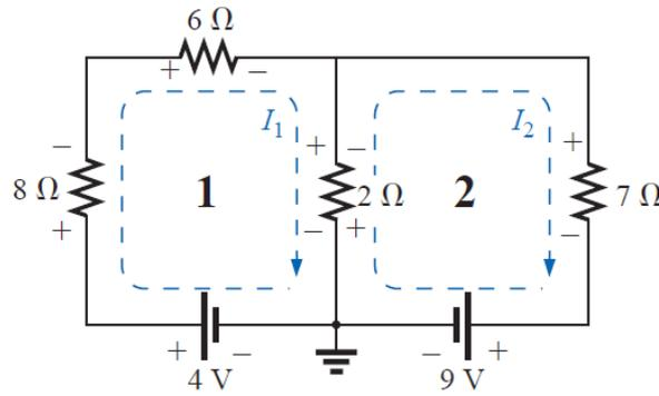
$$I_1: (8\ \Omega + 6\ \Omega + 2\ \Omega)I_1 - (2\ \Omega)I_2 = 4\ \text{V} \quad \text{from loop 1}$$
