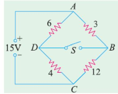
$$R_T = 6 \parallel 3 + 4 \parallel 12 = \frac{6 * 3}{6 + 3} + \frac{4 * 12}{4 + 12} = 5 \Omega \rightarrow I_T = \frac{15}{5} = 3A$$
