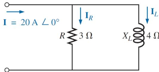
$$I_R = \frac{Z_L I_T}{Z_R + Z_L} = \frac{(4 \Omega \angle 90^\circ)(20 \text{ A} \angle 0^\circ)}{3 \Omega \angle 0^\circ + 4 \Omega \angle 90^\circ} = \frac{80 \text{ A} \angle 90^\circ}{5 \angle 53.13^\circ}$$
