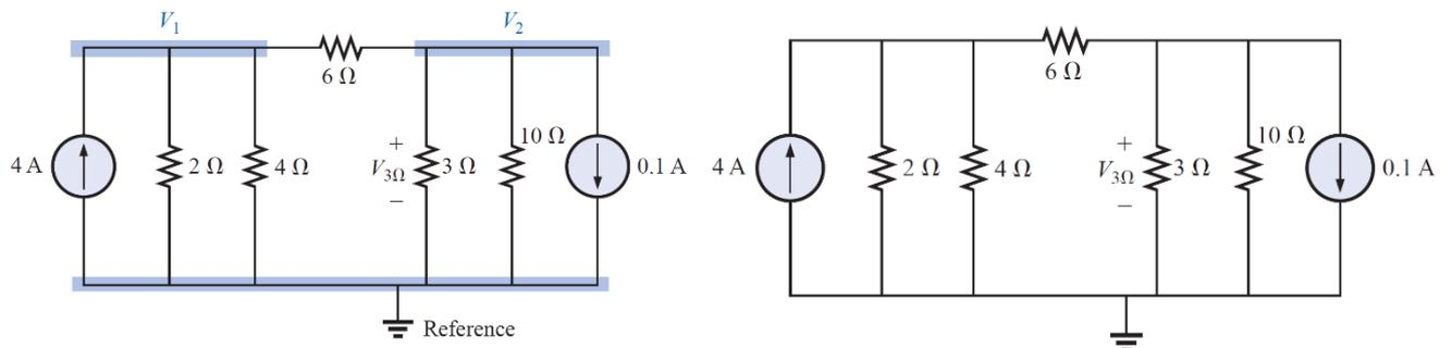
$$\left. \begin{array}{l} \text{Node1: } \left( \frac{1}{2\Omega} + \frac{1}{4\Omega} + \frac{1}{6\Omega} \right) V_1 - \left( \frac{1}{6\Omega} \right) V_2 = +4 \text{ A} \\ \text{Node2: } \left( \frac{1}{10\Omega} + \frac{1}{3\Omega} + \frac{1}{6\Omega} \right) V_2 - \left( \frac{1}{6\Omega} \right) V_1 = -0.1 \text{ A} \end{array} \right\} \rightarrow \begin{array}{l} \frac{11}{12} V_1 - \frac{1}{6} V_2 = 4 \\ -\frac{1}{6} V_1 + \frac{3}{5} V_2 = -0.1 \end{array}$$
