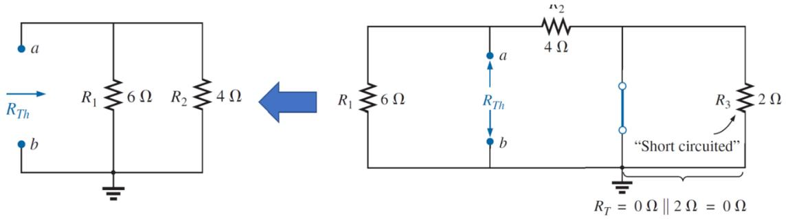
$$R_{Th} = R_1 \parallel R_2 = \frac{(6 \Omega)(4 \Omega)}{6 \Omega + 4 \Omega} = 2.4 \Omega$$
