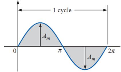
$$v_{av} = \frac{\int_0^{2\pi} A_m \sin t dt}{2\pi} = \frac{-A_m [\cos t]_0^{2\pi}}{2\pi} = \frac{-A_m (1 - 1)}{2\pi} = 0 v$$
