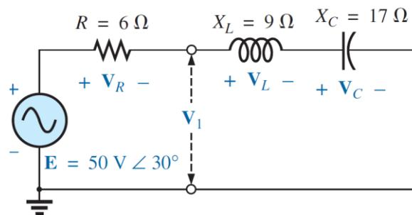
$$V_L = \frac{Z_L E}{Z_T} = \frac{(9 \Omega \angle 90^\circ)(50 \text{ V} \angle 30^\circ)}{10 \Omega \angle -53.13^\circ} = \frac{450 \text{ V} \angle 120^\circ}{10 \angle -53.13^\circ} = 45 \text{ V} \angle 173.13^\circ$$
