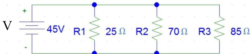
$$\frac{1}{R_e} = \frac{1}{R_1} + \frac{1}{R_2} + \frac{1}{R_3}$$
