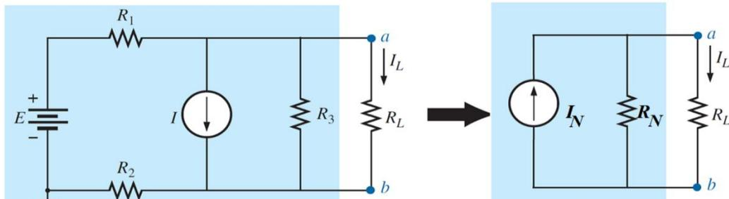
$$I_L = \frac{I_N R_N}{R_N + R_L}$$
