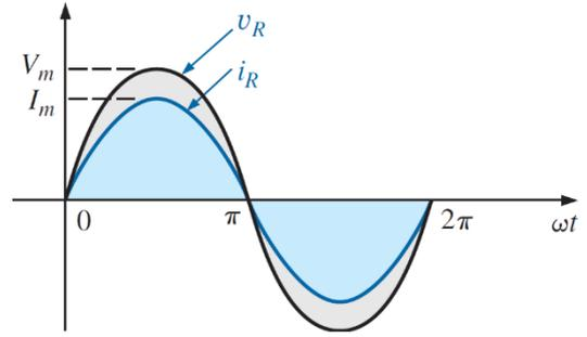
$$P = \frac{V_m I_m}{2} = V_{\text{rms}} I_{\text{rms}}$$
