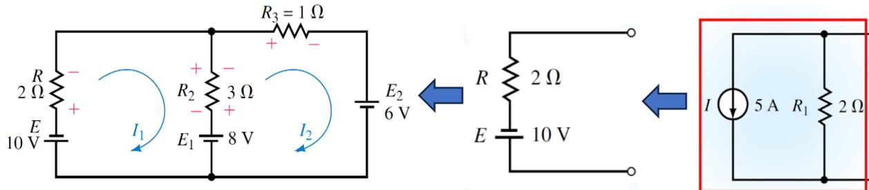
$$\text{Loop 1:} \quad -10\ \text{V} - (2\ \Omega)I_1 - (3\ \Omega)I_1 + (3\ \Omega)I_2 - 8\ \text{V} = 0$$
