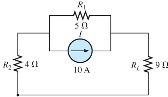
$$R_N = R_1 + R_2 = 5 \Omega + 4 \Omega = 9 \Omega$$
