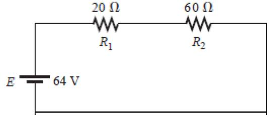
$$V_1 = \frac{64 * 20}{20 + 60} = 16 \text{ v} \quad V_2 = \frac{64 * 60}{20 + 60} = 48 \text{ v}$$
