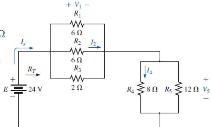
$$I_s = \frac{E}{R_T} = \frac{24 \text{ V}}{6 \Omega} = 4 \text{ A}$$
