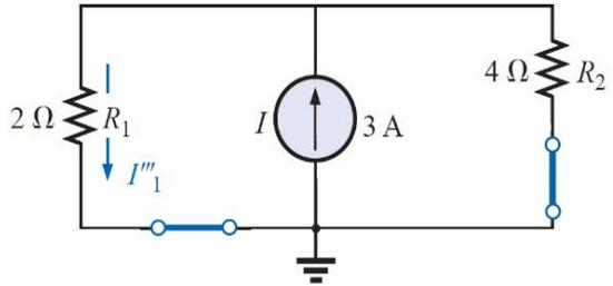
$$I_1 = I''_1 + I'''_1 - I'_1 = 1 \text{ A} + 2 \text{ A} - 2 \text{ A} = 1 \text{ A}$$
