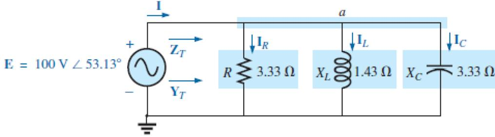
$$Y_T = Y_R + Y_L + Y_C = \frac{1}{3.33 \Omega} \angle 0^\circ + \frac{1}{1.43 \Omega} \angle -90^\circ + \frac{1}{3.33 \Omega} \angle 90^\circ$$
