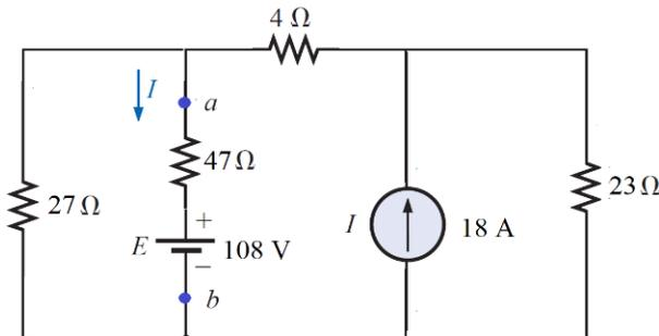
$$R_{Th} = (4\Omega + 23\Omega) \parallel 27\Omega$$
