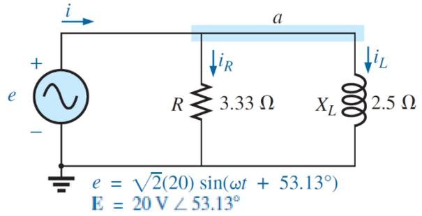
$$I_R = \frac{E \angle \theta}{R \angle 0^\circ} = (20 \text{ V} \angle 53.13^\circ)(0.3 \text{ S} \angle 0^\circ) = \mathbf{6 \text{ A} \angle 53.13^\circ}$$
