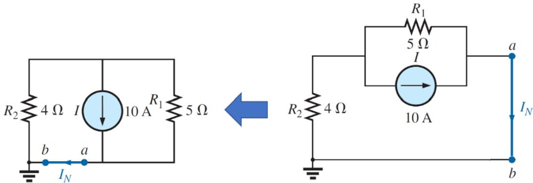
$$I_N = \frac{R_1 I}{R_1 + R_2} = \frac{(5 \Omega)(10 \text{ A})}{5 \Omega + 4 \Omega} = \frac{50 \text{ A}}{9} = 5.56 \text{ A}$$
