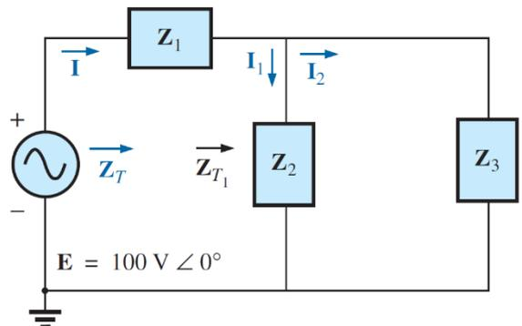
$$\begin{aligned} Z_T &= Z_1 + Z_{T_1} \\ &= 4 \Omega + 6.68 \Omega + j 0.28 \Omega \\ &= 10.68 \Omega + j 0.28 \Omega = \mathbf{10.68 \Omega \angle 1.5^\circ} \end{aligned}$$
