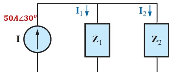
$$\begin{aligned} \mathbf{I} &= \mathbf{I}_1 + \mathbf{I}_2 \\ 50 \text{ A } \angle 30^\circ &= 80 \text{ A } \angle -6.87^\circ + 50 \text{ A } \angle 136.26^\circ \\ &= (79.43 - j 9.57) + (-36.12 + j 34.57) \\ &= 43.31 + j 25.0 \\ 50 \text{ A } \angle 30^\circ &= 50 \text{ A } \angle 30^\circ \end{aligned}$$
